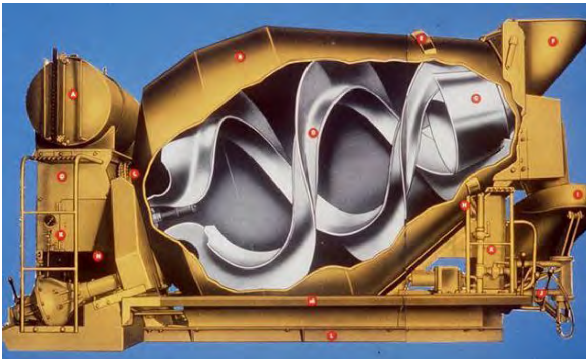
Figure 4-13 Cut-Away View of Transit Mix Drum
