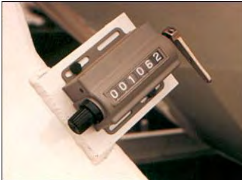
Figure 4-17 Mechanical-Arm Revolution Counter
