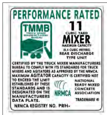
Figure 4-14 TMMB Discharge Rating Plate 1
