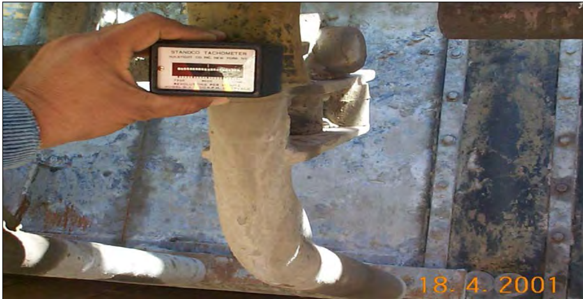
Figure 4-98 Optical Wedge Sicker for Measuring Vibrator Amplitude
