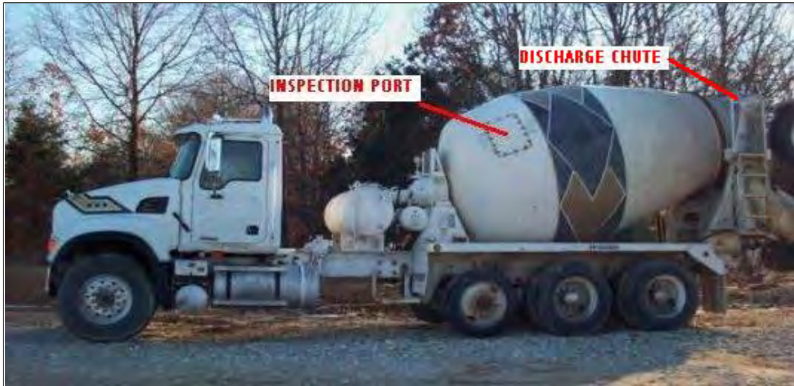
Figure 4-16 Inspection Port on Inclined-Axis Revolving Drum
