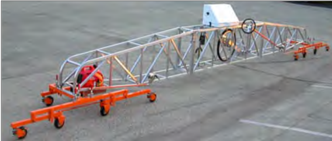
Figure 4-123 California Profilograph (Note Measuring Wheel in Center of Frame is Retracted for Transporting)
