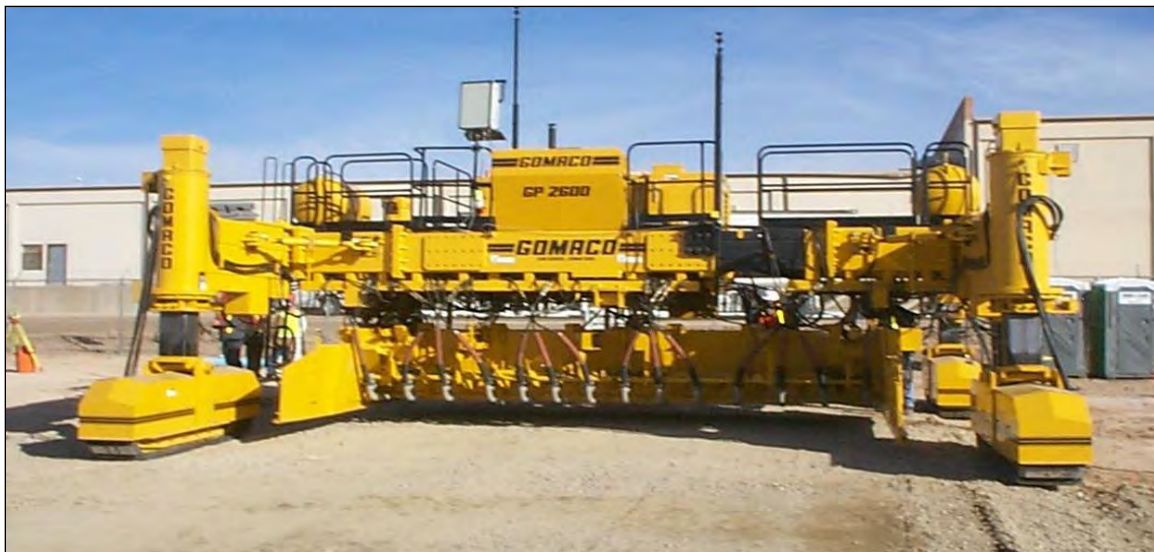
Figure 4-78 Typical Slipform Paver, Showing Vibrators and Knock-Down Auger (Note Unstable Base Course Under the Right Tracks of the Paver)
